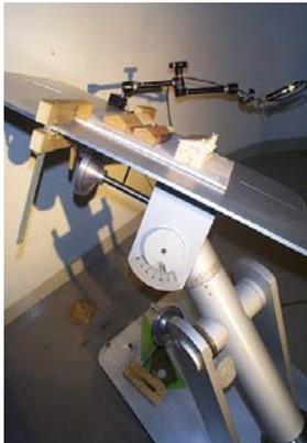
A Heliodon simulates solar exposure and shading
